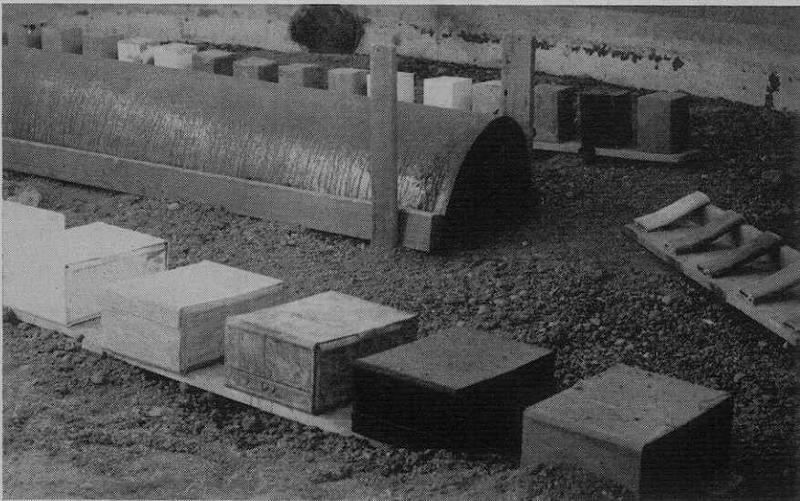
Figure 3. Evaluation of rodent resistance of test carbons and other materials under exposure station conditions
